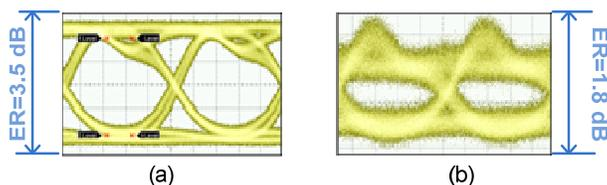
Fig. 5. Eye diagrams of upstream directly modulated signal (a) original 10 Gb/s upstream signal (b) SOA amplified 10 Gb/s upstream signal.
