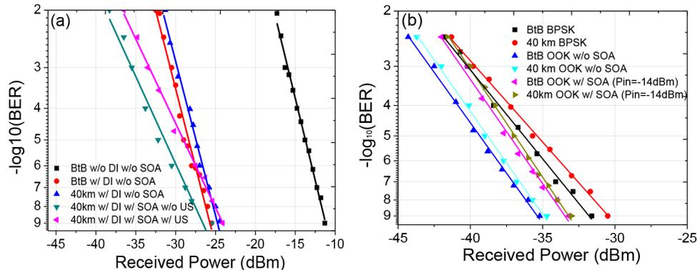
Fig. 4. BER curves of downstream (a) and upstream (b) signals.
